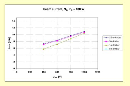
Beam current in dependence from the extraction voltage
