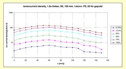
*lon current density profile (at logarithmic scale) 50 mm from the ECR plasma source, (1.5x10-3mbar nitrogen, 40W)*
