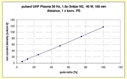
Maximum ion current density at 50 mm from the ECR plasma source, (1.5x10-3mbar nitrogen, 40W)
