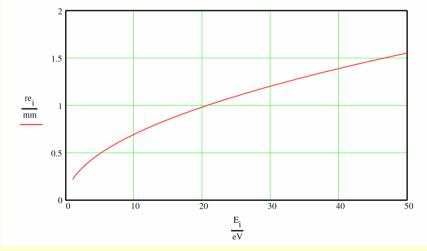
Typical electron radius for ECR conditions at 433 MHz
