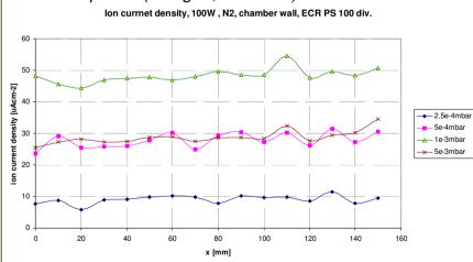
Ion current density at the chamber wall in dependence from the pressure (nitrogen, 100 W)
