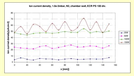
Ion current density at the chamber wall in dependence from UHF power (nitrogen, 10<sup>-3</sup>mbar)
