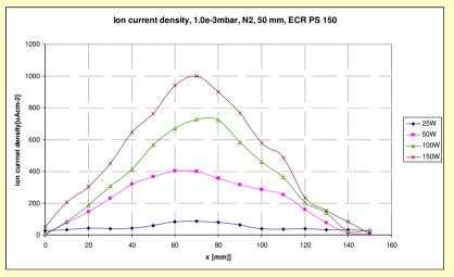
Ion saturation current density profile at 50 mm distance
