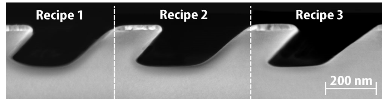
Control of parallelism with different etching conditions for SiO 2
