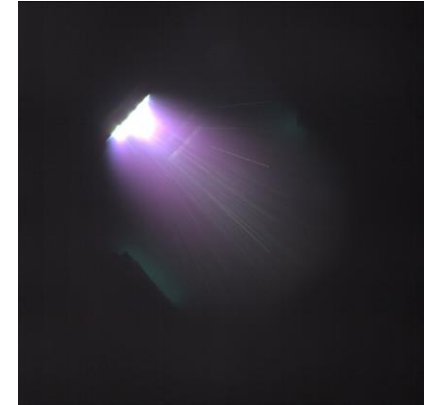
Arc discharge of the laser-arc module (LAM)
