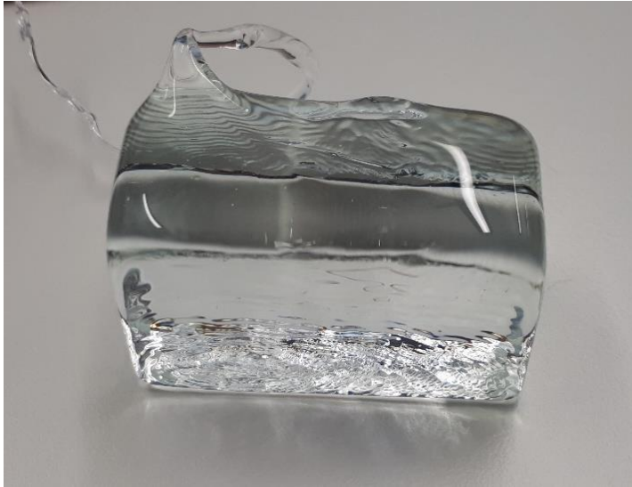
85 SiO 2 - 15 Rb 2 O glass made at 1600 °C
